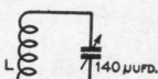
Figure 2. Nothing could be simpler than the circuit of an absorption type wavemeter. For the range of from 8 to 30 meters, L should consist of 8 turns 1" long on a 1 1/4"-diameter form. For 30 to 95 meters, L should consist of 27 turns 1" long on a 1 1/4"-diameter form.
