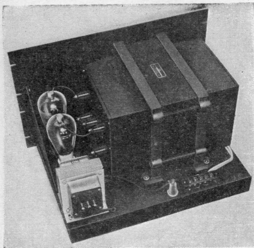
Figure 31. The heavy-duty high-voltage power transformer and the rectifiers are mounted on the bottom rack.
