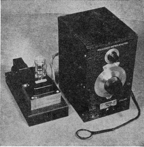
Figure 36. This conversion exciter was built in the same cabinet as a combined frequency meter and monitor, both obtaining power from the external supply shown to the left.
